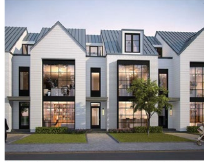
Fig. 3.47 A combination of Upper Story Stepbacks and visible sloped roofs can provide rooftop variety and reinforce building massing.
